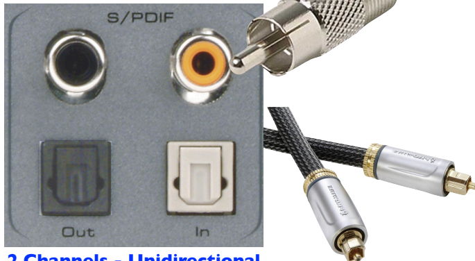
2 Channels - Unidirectional RCA connectors with coaxial cable Toslink Connectors - Optical cable
